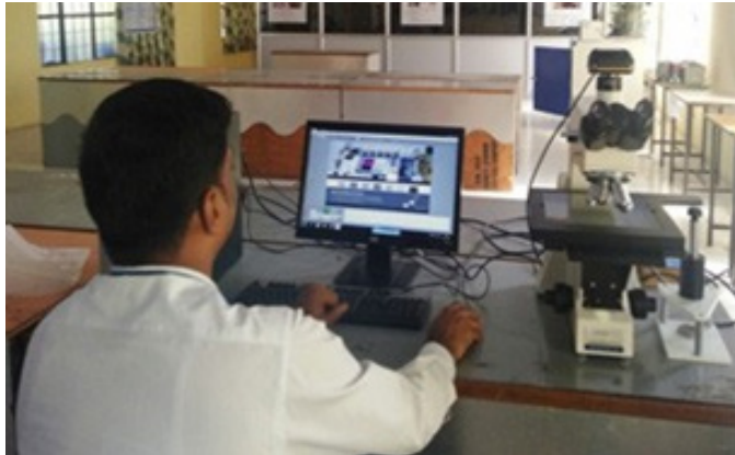
Optical Microscope with Data Acquisition System
